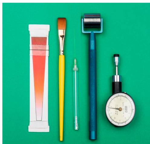
Figure 1. The test instruments summarised in Table 2: Coloured Analogue Scale, Camel hair brush, von Frey optical glass filament No 12, ThermoRoll (at 22 °C), Fischer Handheld Pressure Algometer. The sources are in Supplementary Table S3.
